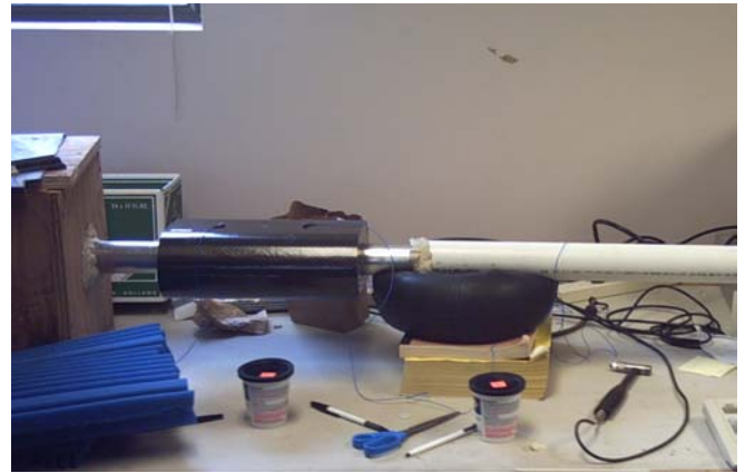
Figure 19. Vibration and acoustic test setup, showing the acoustic source in an acoustically isolated box (at left of picture).
